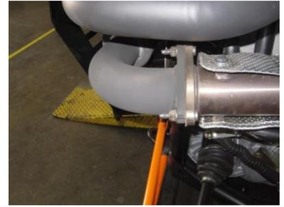
2. Once you have removed the heat shield remove the factory brackets and re install the Gibson supplied brackets #E using the factory bolts and factory location. Keep loose until final install.
