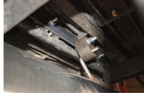
Install the hanger bracket using the supplied bolt kit. This bracket will also support the supplied rubber grommet.
