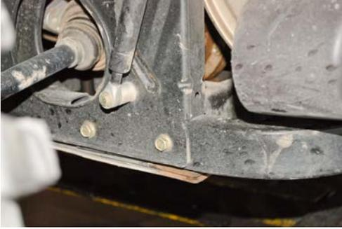
Begin the removal of the factory exhaust by removing the factory hitch; there are a total of four bolts two on each side. Removing the factory skid plate will make for an easier removal of the hitch but is not a necessary step.
