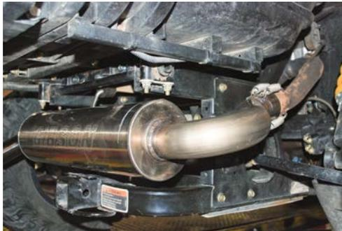
Use the factory gasket and springs for the install of the Gibson exhaust.
